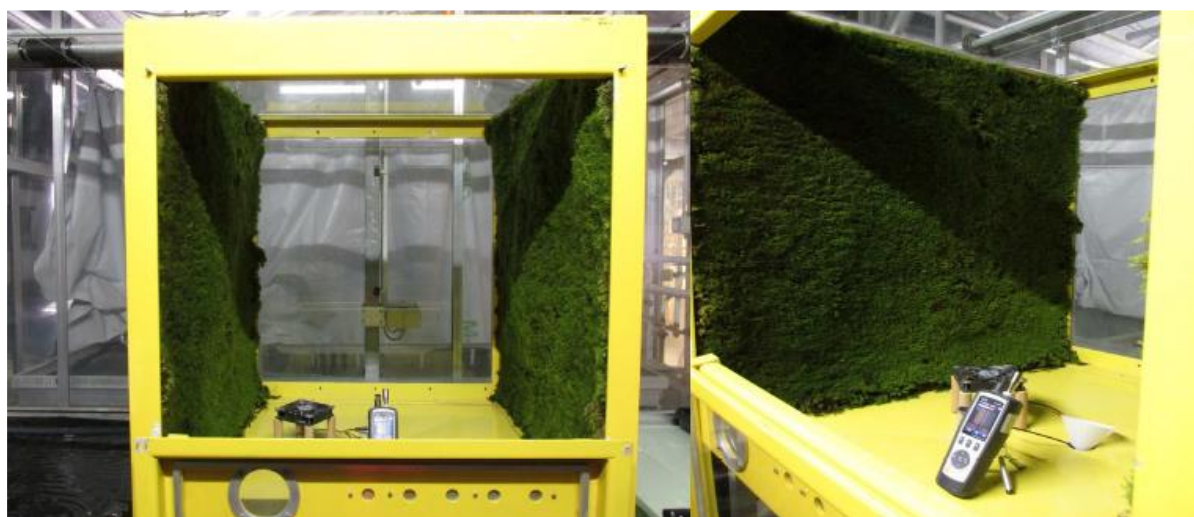
Fig. 1: Model with mossmats and technical equipment
