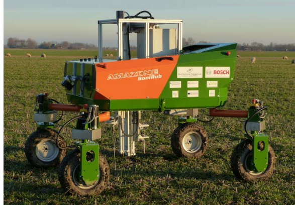
Fig. 2. BoniRob with Penetrometer App during field trails in the Netherlands
