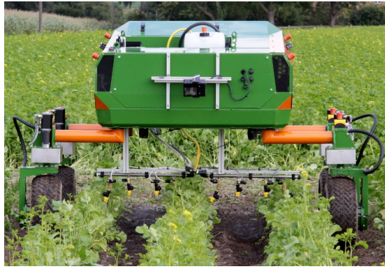
Figure 2: BoniRob with Precision Spraying App during field test
