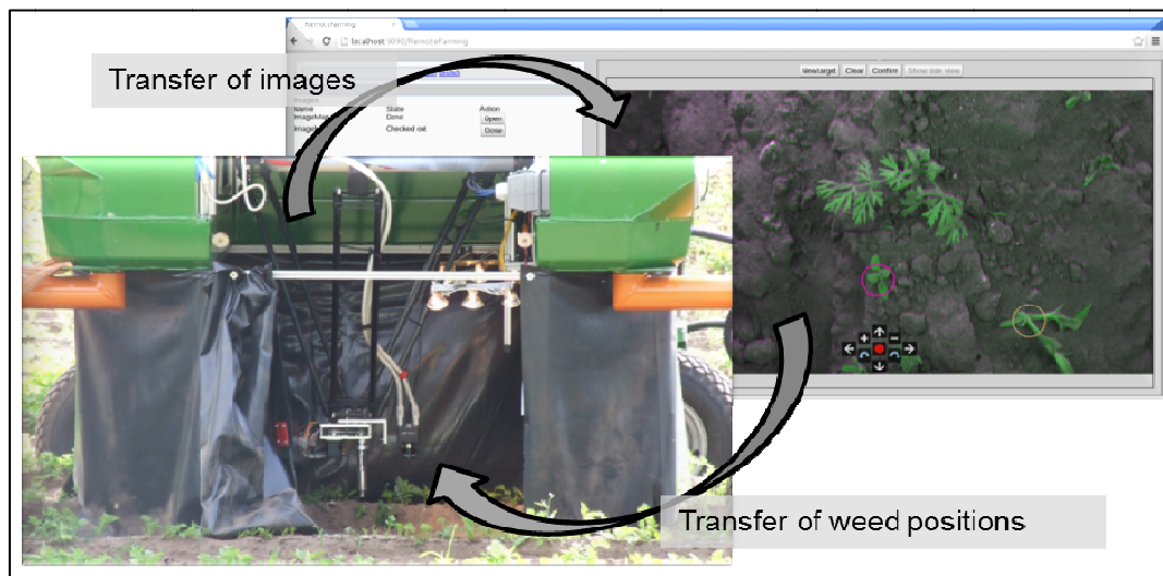
Fig. 6: Web-based communication between the mechanical weed control system and the remote worker's web client GUI
