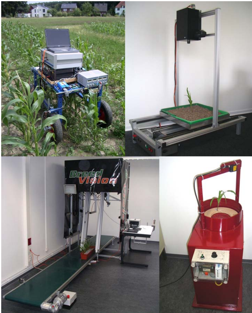
Fig. 9 Experimental test setups for plant measurements: Outdoor test vehicle (top left), powered spectral imaging setup (top right), powered conveyor belt system (bottom left) and powered high-speed carousel (bottom right).
